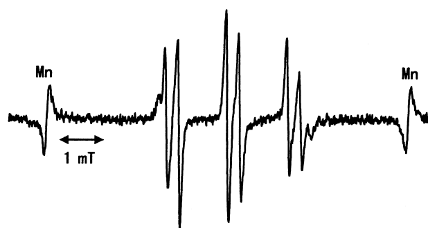
Figure 2. ESR spectra of PBN adducts obtained from the DMSO/H 2 O 2 /NaOH system.
